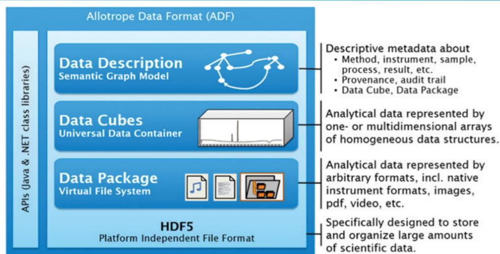
Figure 2: Allotrope Data Format (ADF) Overview
